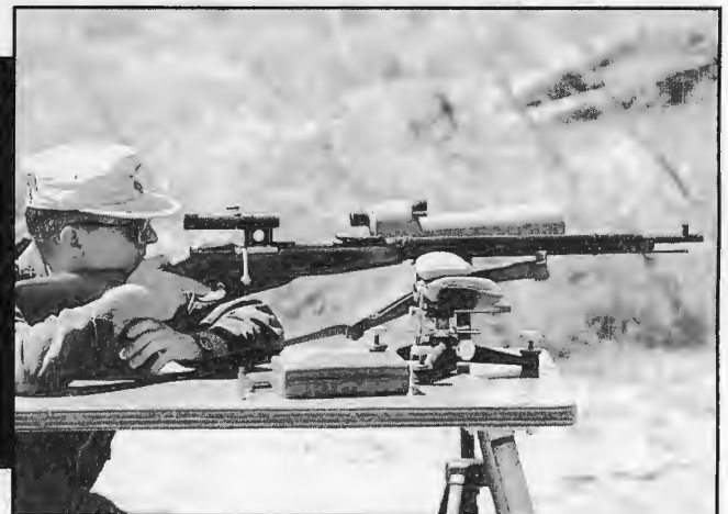
Shooting the Mosin-Nagant M1891/30 sniper rifle from a benchrest with standard military ball ammunition of three types produced accuracy no better than 2.3 MOA at 100 yards.
